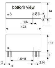
All dimension in mm, tolerance: .x±0.5mm]
