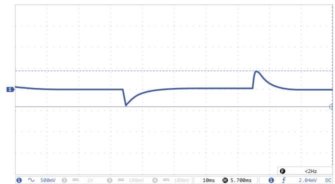
Figure 8 (d). Oscilloscope chart of voltage transient deviation during load “drop/rise”.
