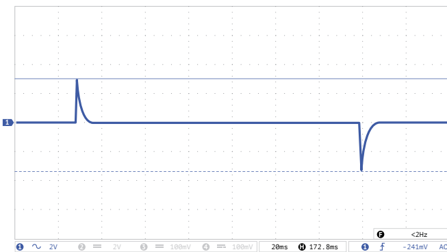
Figure 8 (d). Oscillograph chart of voltage transient deviation during load “drop/rise”.
