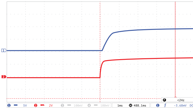
Figure 7 (a). Oscillograph chart of setting output voltage after supplying remote control signal to ON-output.
