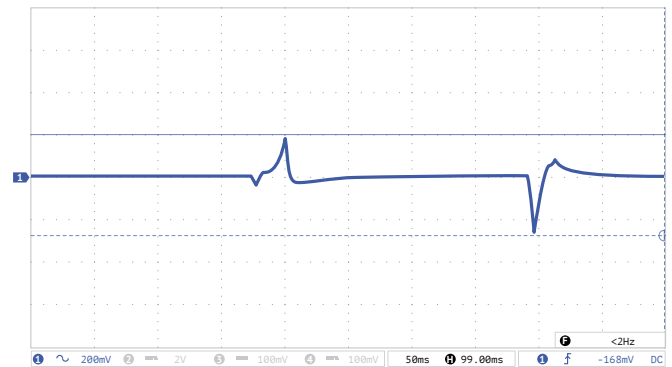
Figure 7 (d). Oscillograph chart of voltage transient deviation during load "drop/rise".
