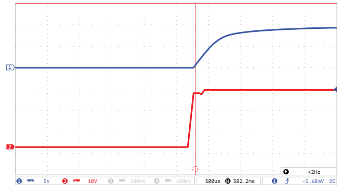
Figure 7 (b). Oscillograph chart of output voltage after supplying the input voltage.
