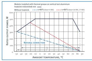
Decreasing parts of the dashed and dash-dotted curves correspond to the maximum case temperature (+85°C for models with index «N» and «P»). Output power must not exceed the values limited by curve for a given ambient temperature.
