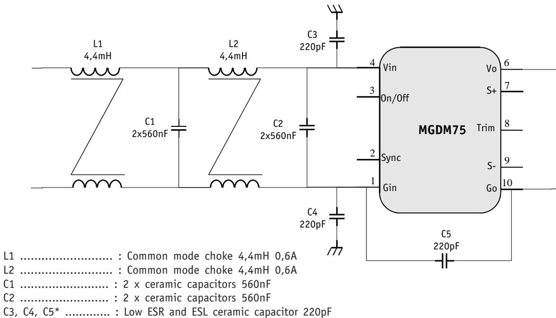
(\*) Must be placed as close as possible to the converter in order to reduce the path length or the connections to the pins and the baseplate.
